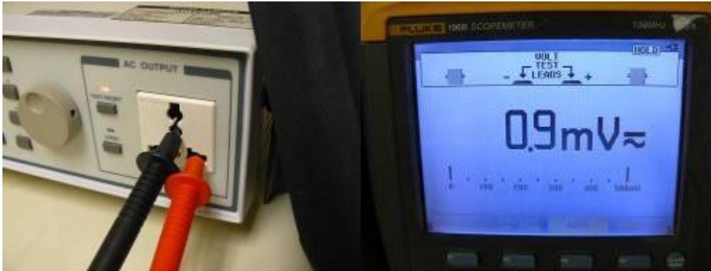
*Figure 6c: Voltage measurement between neutral and ground with neutral tied to ground reference.*
